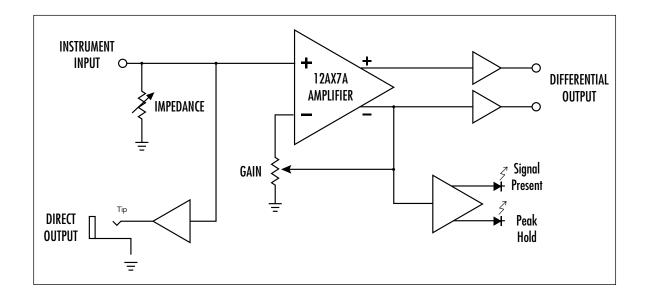
The Instrument Input to the TD-100 is directly connected to the Direct Output. The Impedance control sets the input impedance of the first stage input. The Impedance control can be used to match the impedance of the instrument and to provide subtle tonal coloration.
